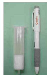
Presep® Syringe Type with one end open
